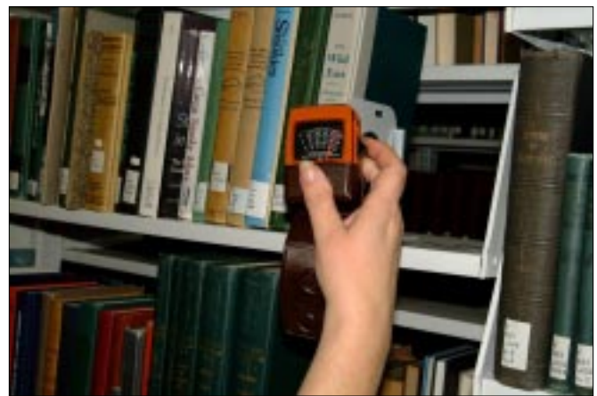
Taking a light reading in the stacks. Light and heat embrittle paper.
